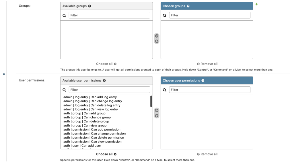
Figure 5.2: User object view in Django Admin showing all the groups and user permissions attached to the given user
